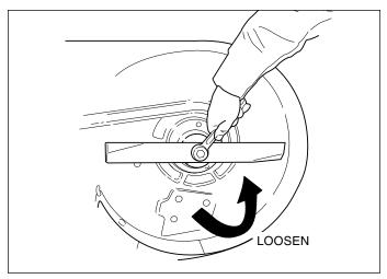
Figure 7. Removing the Blade
